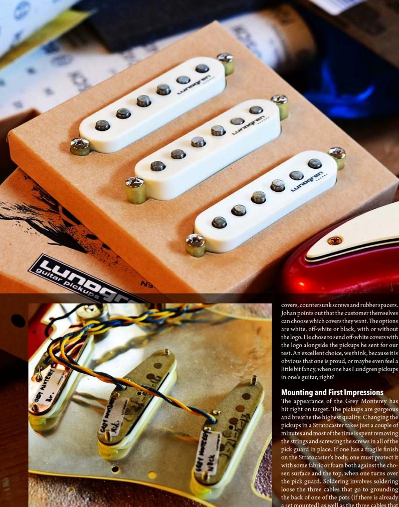
A good tip can be to twist the connection cables to minimise humming.
